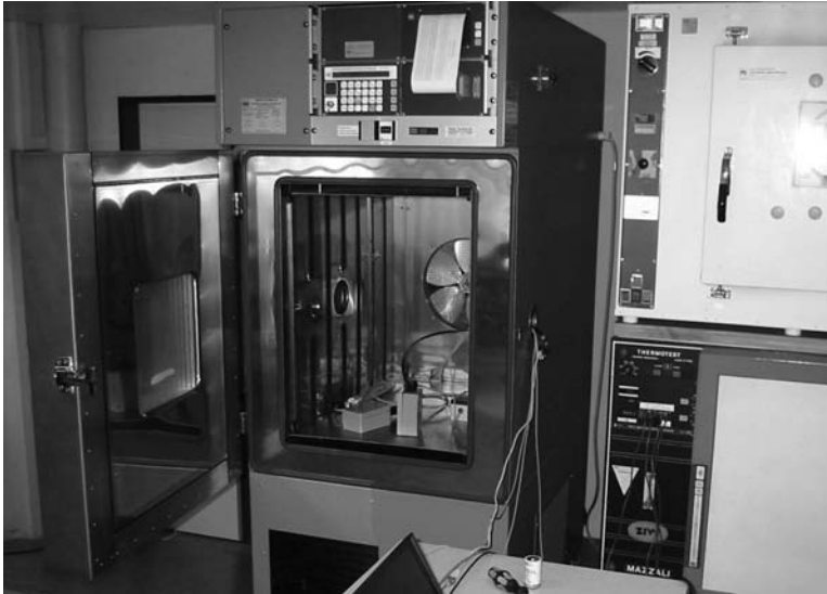
FIGURE 11.12 TCT chamber for emulating harsh environmental conditions.
