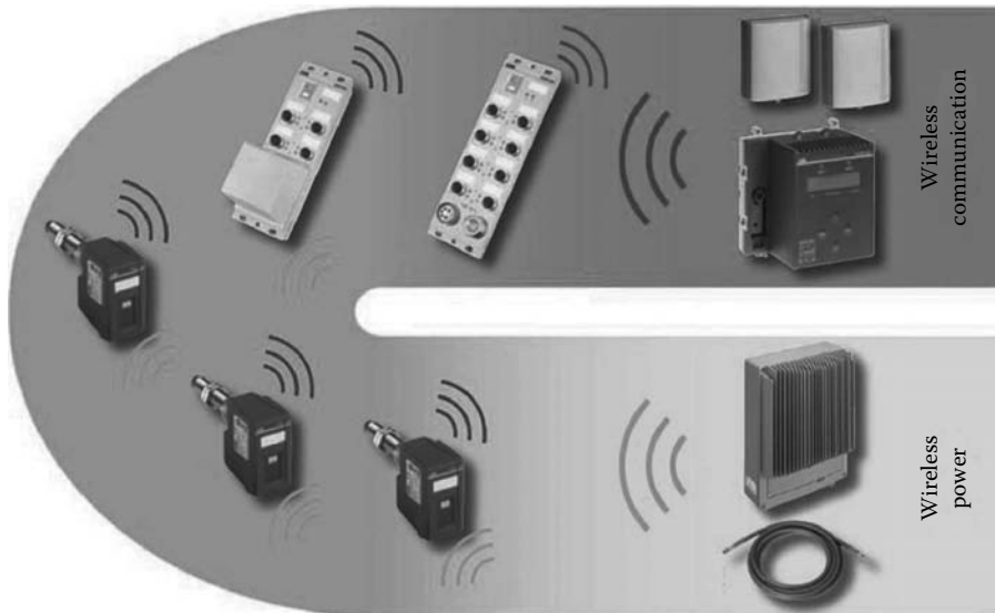
FIGURE 28.15 Industrial automation devices with embedded WISA-POWER and WISA-COM technologies (left side) and necessary infrastructure (right side).
