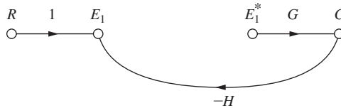
FIGURE 5-5 Original flow graph for the sampled-data system in Fig. 5-4.
