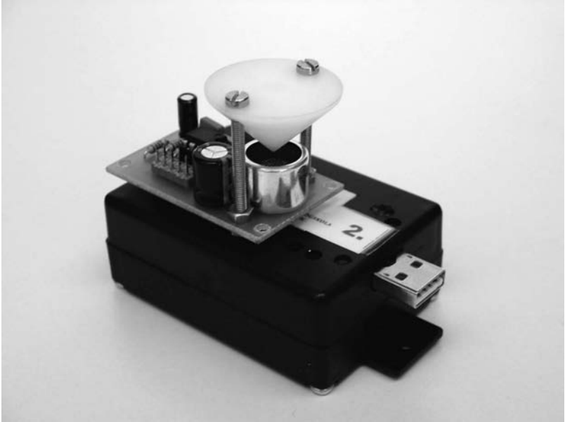
FIGURE 6.11 Stationary sensor network nodes with ultrasound receiver circuit. The node is packaged in a plastic box to reduce wear.
