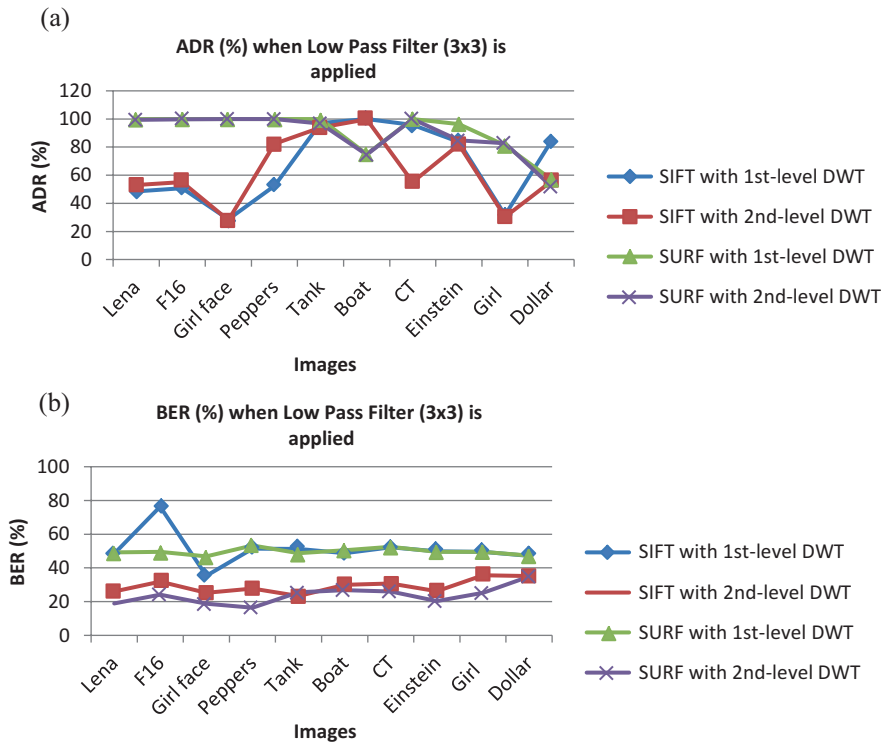
Fig. 3.24 Performance comparison in terms of (a) ADR and (b) BER when low pass filter (3 × 3) is applied
