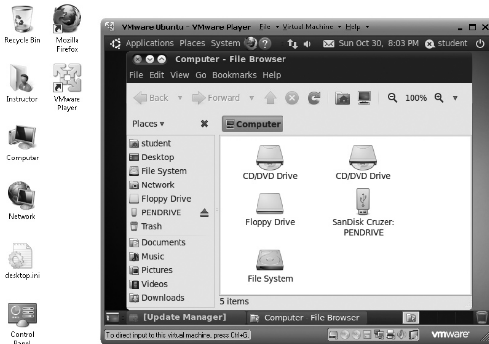
FIGURE 17-5 Ubuntu running in a VMware Player virtual machine on Windows 7. Note the flash drive icon.
