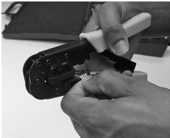
FIGURE 4-2 Aligning the wires and evening the ends
