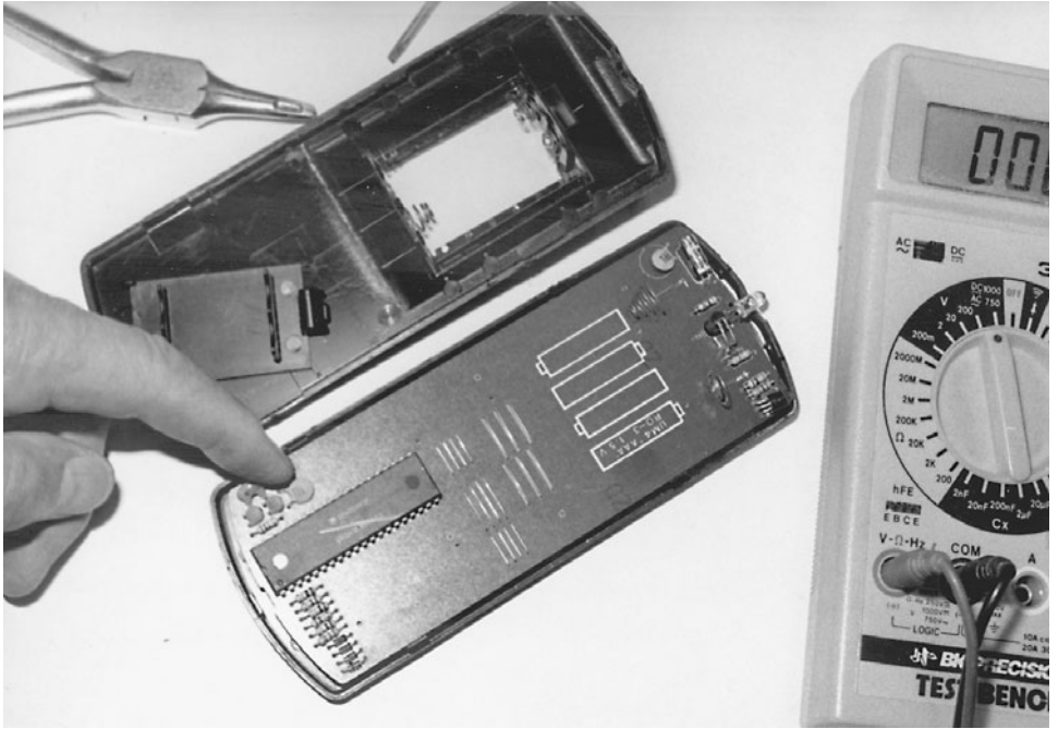
12-3 Suspect weak batteries when remote operation is intermittent or the remote must be close to the electronic product to function.
