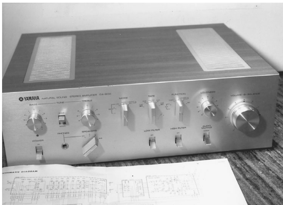
9-18 Check all electrolytic capacitors within the high-powered transistor stereo amplifier with an ESR meter.
