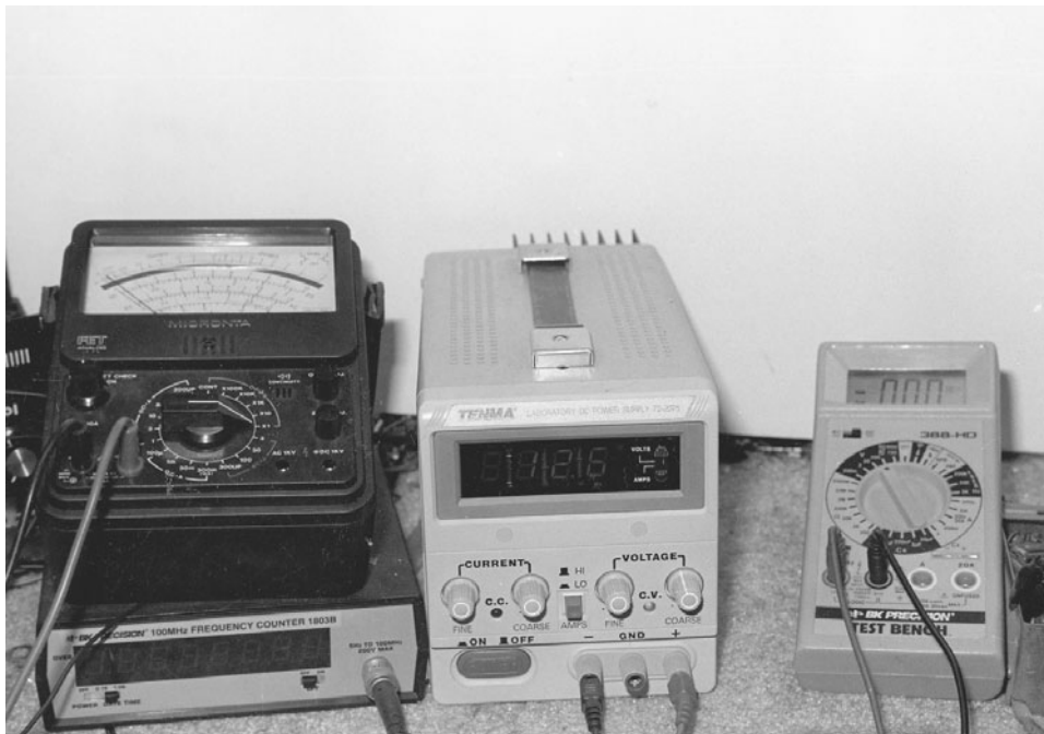
3-1 A good VOM or DMM can quickly locate a defective part within an electronic chassis.
