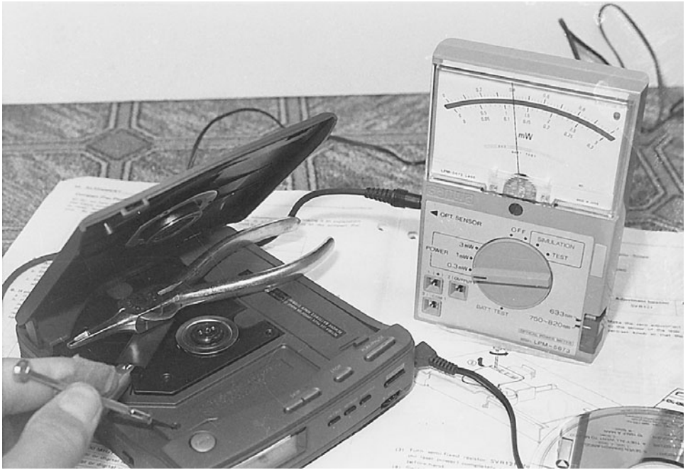
6-5 Check the laser diode lens assembly with a laser power meter.
