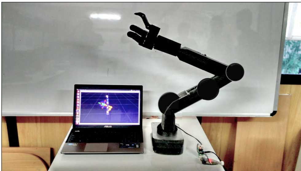
Figure 16 : COOL-Arm-5000 prototype with MoveIt! visualization
