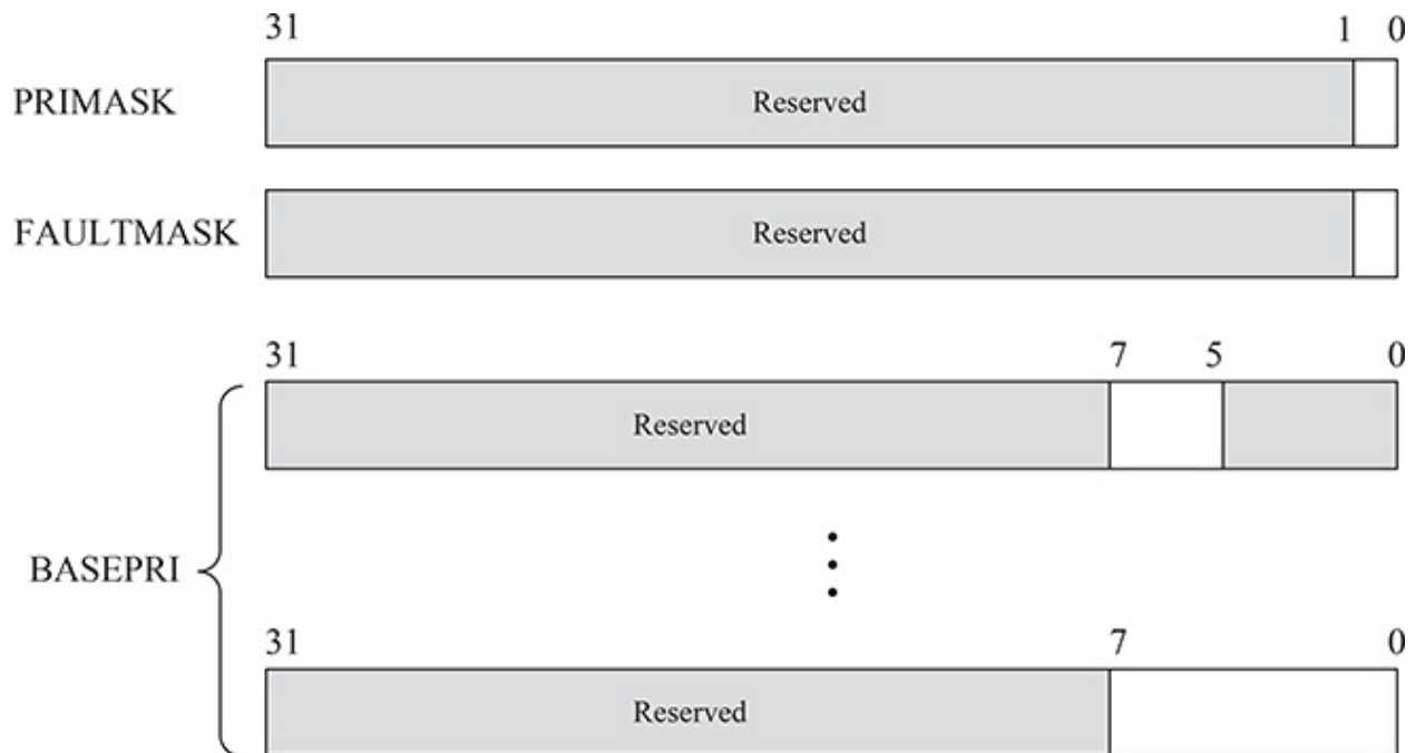
Figure 3.4: Registers used for interrupt masking. For the BASEPRI register two extreme scenarios corresponding to 3-bit and 8-bit implementation are shown.
