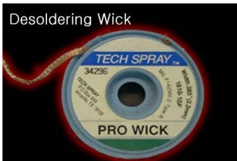
Close up to a piece of solder wick
