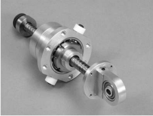
Figure 6 A ballscrew inerter made in the University of Cambridge engineering department in 2003, with flywheel removed.
