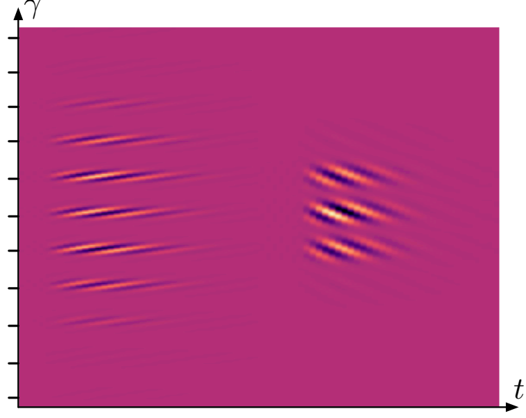
Figure 4.11: Spiral wavelets in the time-frequency domain. Brighter colors denote greater algebraic values of the real part. The background color corresponds to a null real part. Ticks on the vertical axis denote octave intervals.
