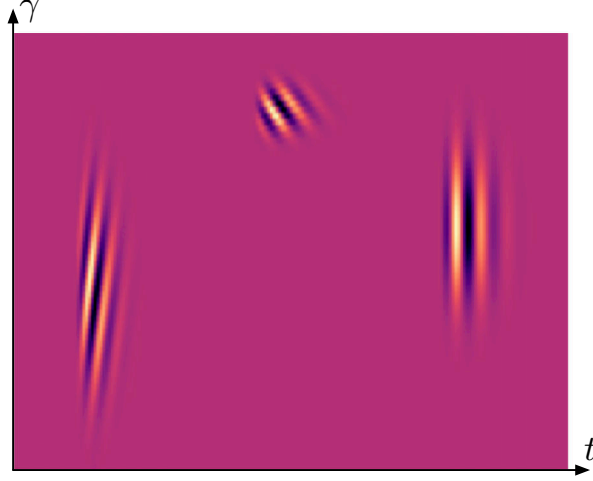
Figure 3.3: Joint time-frequency wavelets in the time-frequency domain. Brighter colors denote greater algebraic values of the real part. The background color corresponds to a null real part.
