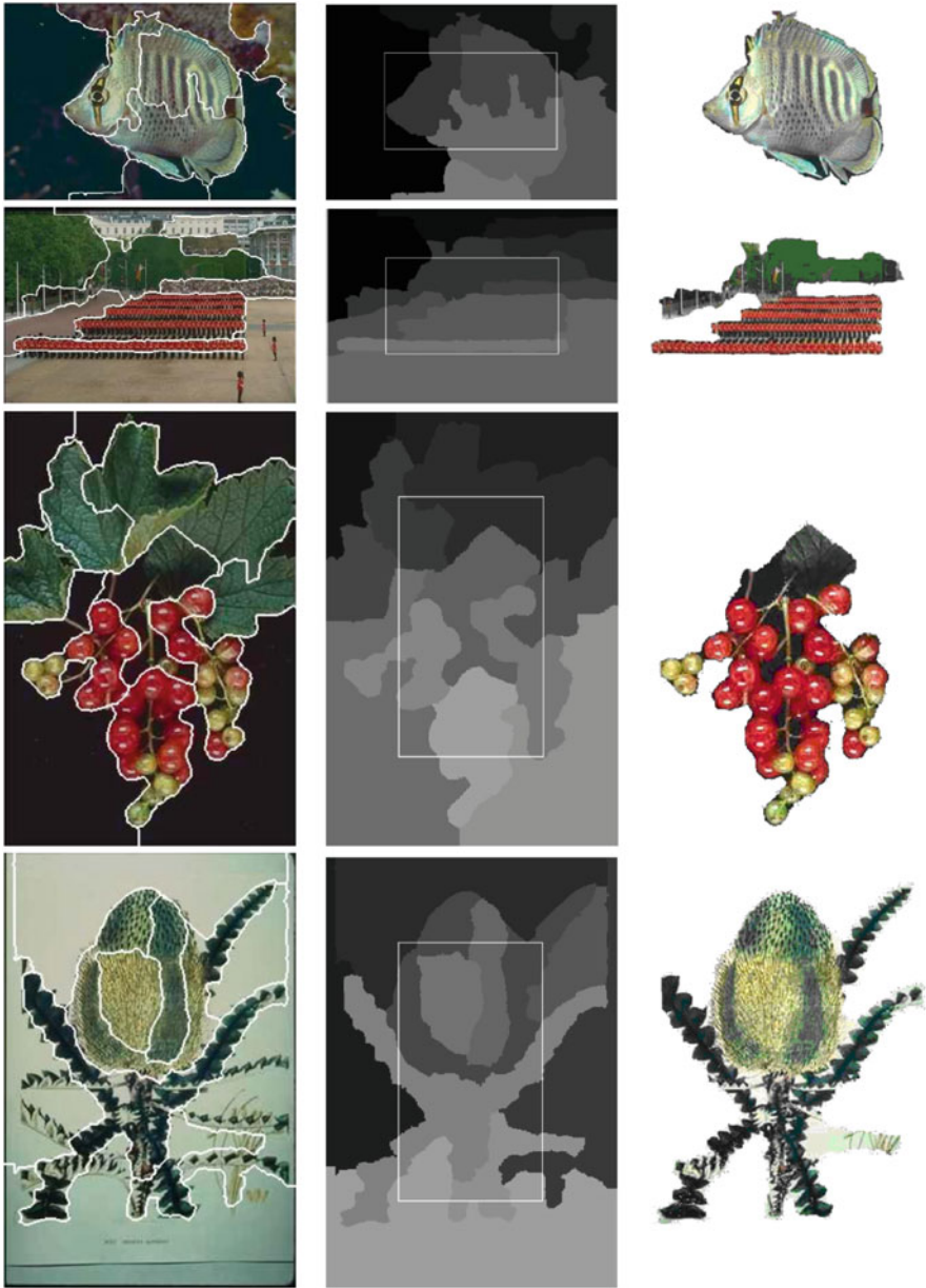
Fig. 3.10 Characterization of region of interest (ROI) using the Edge Flow model inside the W_m \times n window. Left column : Edge Flow boundary detection; middle column : ROI identification; and right column : ROI image as the output results
