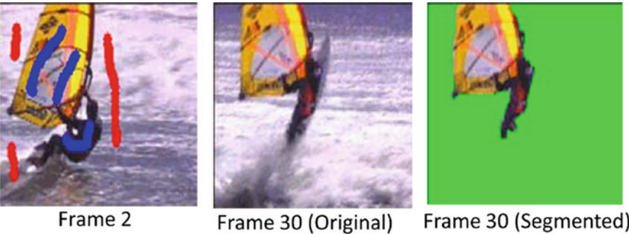
Fig. 7.9 Object segmentation, obtained by user marked objects in Frame 2, and the system automatically tracks and segments the objects until Frame 30
