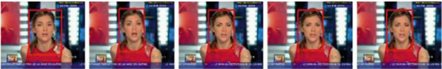
Fig. 7.19 Face detection result obtained by the application of the trained face detector to the video frames under good illumination
