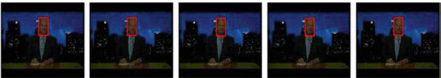
Fig. 7.20 Face detection result obtained by the application of the trained face detector to the video frames under bad illumination
