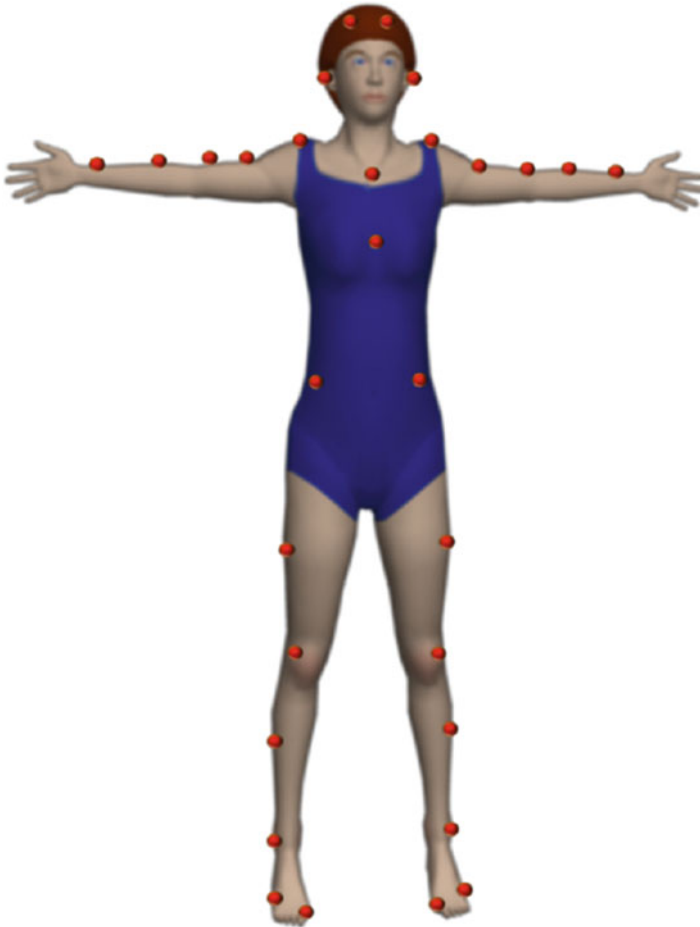
Fig. 11.12 Optical motion capture using retro-reflective markers attached to the actor's body
