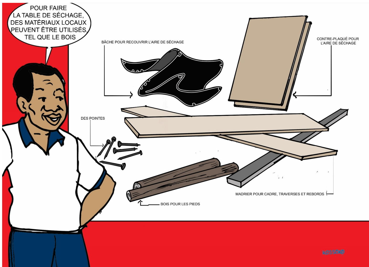
Image 7. Introduction of solution: drying table for parboiled rice paddy, required materials
