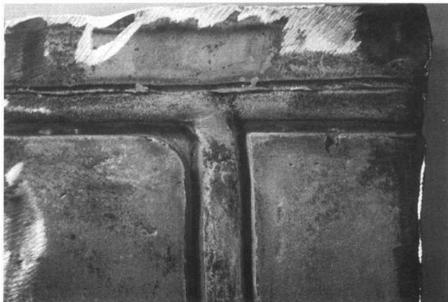
Figure 2-38. Type 316 plate was used here instead of the specified 316L. This is the classic HAZ corrosion of sensitized stainless steel.
