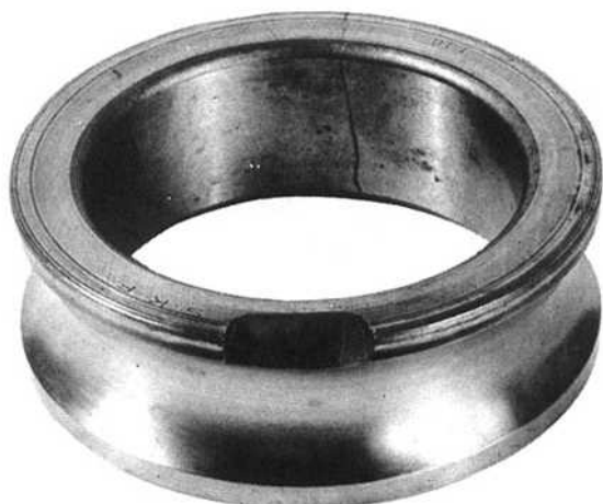
Figure 3-34. Axial cracks caused by an excessive interference fit.
