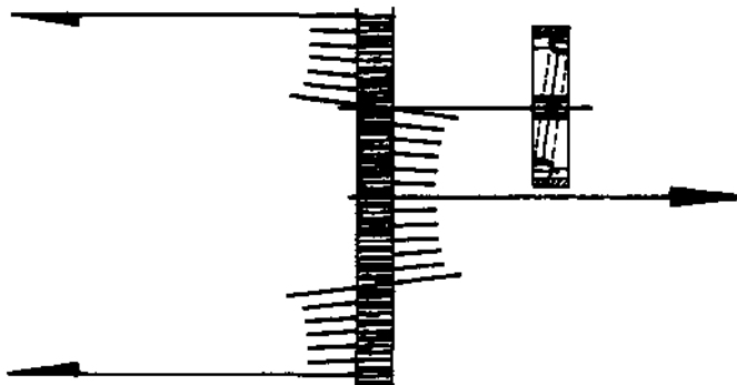
Figure 3-147. Developed plan of an angularly misaligned gear coupling half. 15
