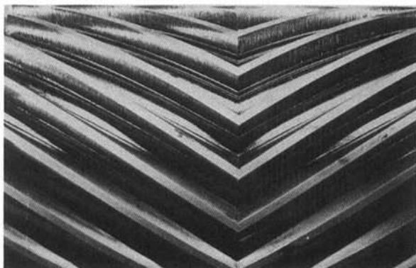
Figure 3-114. Abrasive Wear. This herringbone pinion, nitrided to 42 Rc, shows abrasive wear from foreign particles imbedded in the mating gear.
