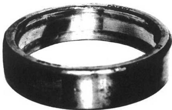
Figure 3-56. False brinelling caused by vibration in the presence of abrasive dirt while bearing was rotating.
