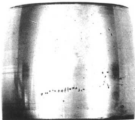
Figure 3-59. Electric pitting on surface of spherical roller caused by the passage of a relatively large current.
