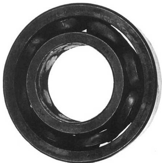
Figure 3-36. Discoloration and softening of metal caused by inadequate lubrication and excessive heat.
