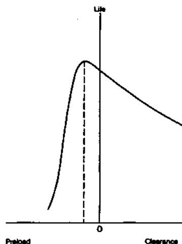
Figure 10-20. Excessive preloads and/or clearances will adversely affect bearing life.
