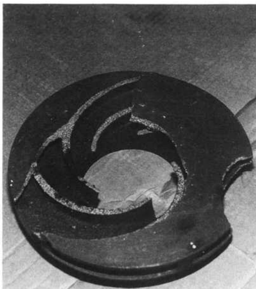
Figure 10-11. Impeller after careless disassembly.
