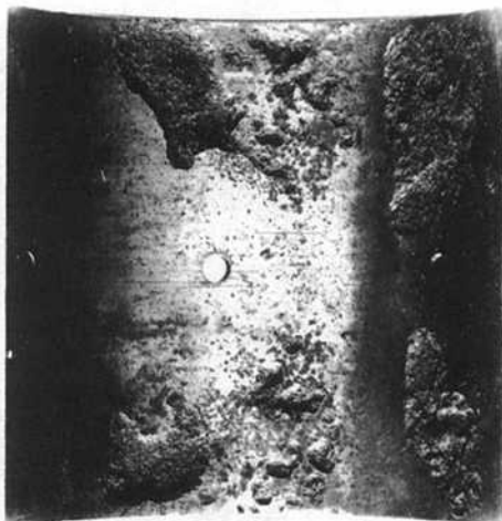
Figure 3-81. Sulphur corrosion of phosphor-bronze bushing.
