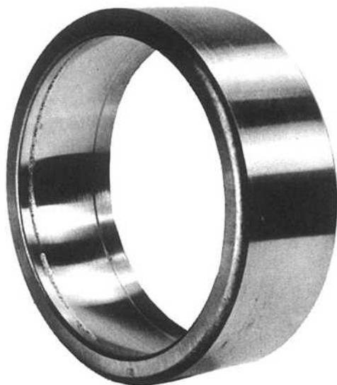
Figure 3-30. Spalling from parasitic thrust.
