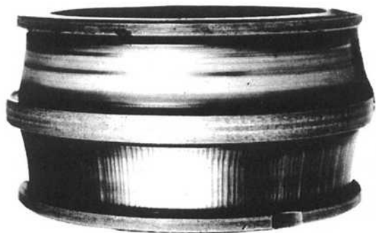
Figure 3-64. Fluting on inner raceway of spherical roller bearing.
