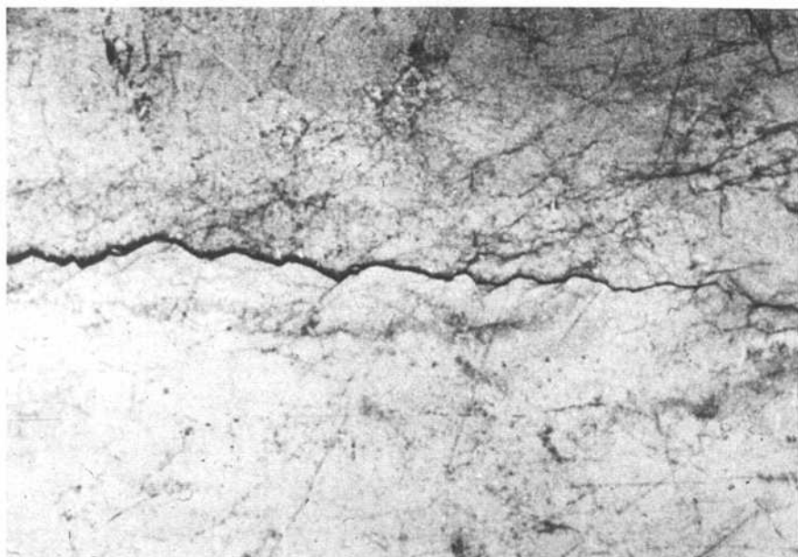
Figure 2-31. Chloride stress corrosion cracking of 316L vessel wall. Reduced 50% from actual size.
