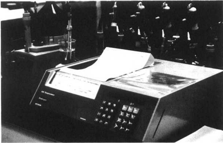
Figure 3-182. Titroprocessor determines total acid number.
