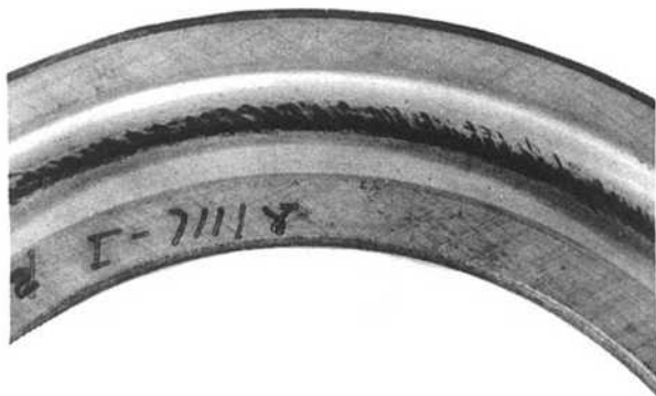
Figure 3-22. Smearing in ball thrust bearing.
