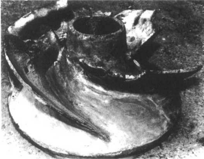
Figure 2-28. Cast-bronze mixed-flow pump impeller failed from cavitation corrosion.
