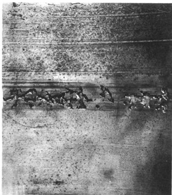
Figure 3-74. Fatigue cracking due to shaft ridging.
