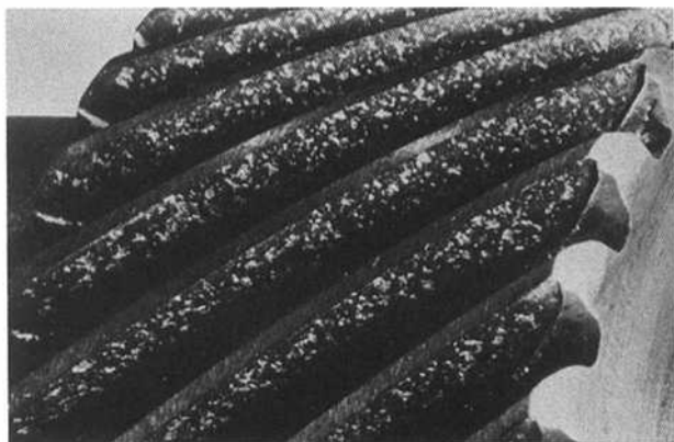
Figure 3-116. Corrosive Wear. It is evident from this gear that considerable wear has taken place yet the surface still shows signs of being attacked chemically. Wear of this nature will continue until the gear surface is completely beyond usefulness.
