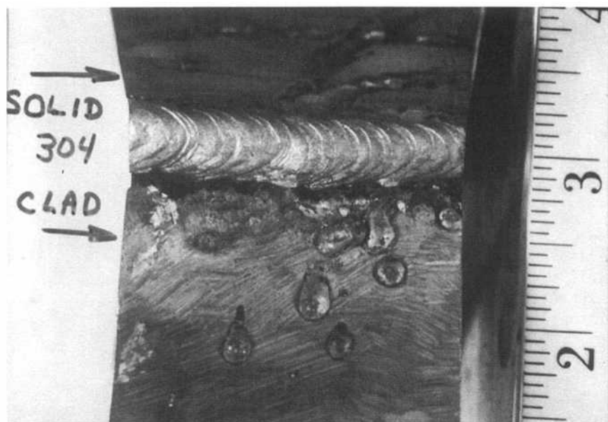
Figure 2-33. The fillet weld between the 304L roof/deck plate and clad 304L wall partition plate. The dark line at the base of the weld on the clad side is undercutting.
