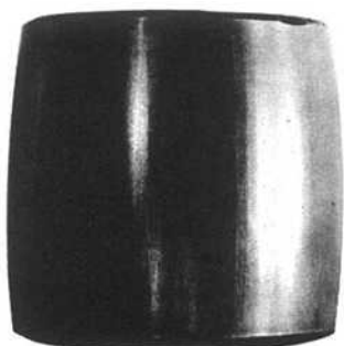
Figure 3-61. Fluting on surface of spherical roller caused by prolonged passage of electric current.
