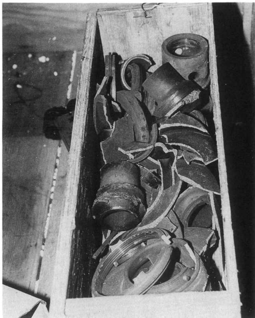
Figure 10-13. Impellers after careless removal from shaft.
