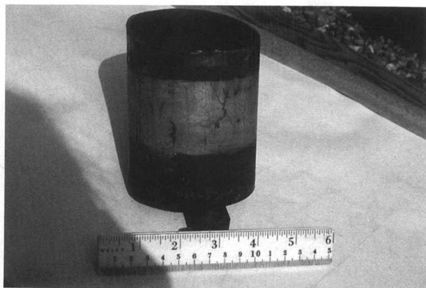
Figure 2-41. This 316L process line failed due to external stress corrosion cracking under a fabricator sticker that was then painted over. Chlorides from the sticker or the atmosphere attacked the unprotected pipe.
