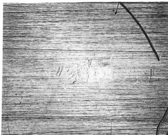
Figure 3-58. Example of false brinelling—100x.
