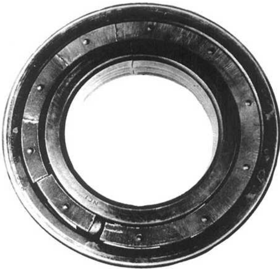
Figure 3-46. Broken cage caused by ineffective lubrication.
