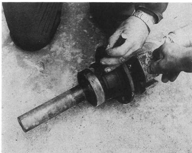
Figure 10-12. Careless disassembly of defective bearing.
