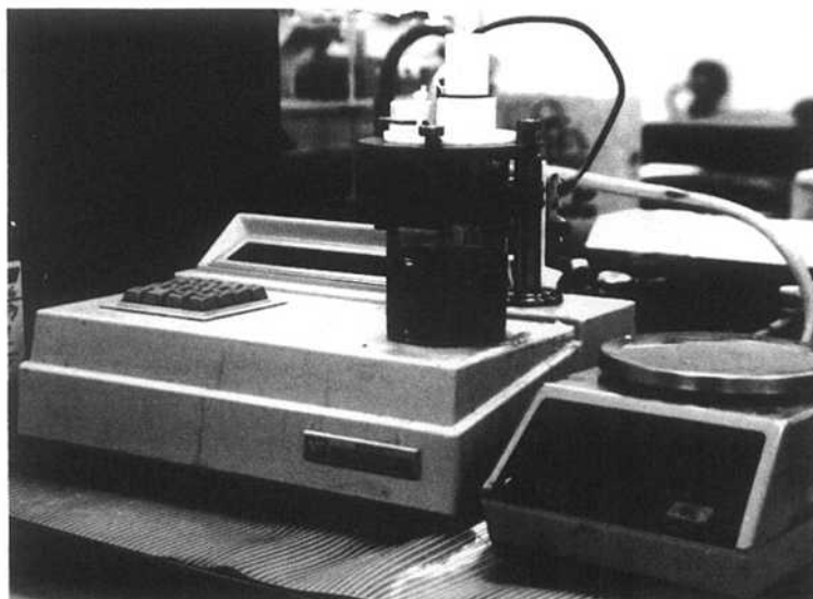
Figure 3-179. Automated titration equipment used to test for dissolved water (Karl Fischer method).
