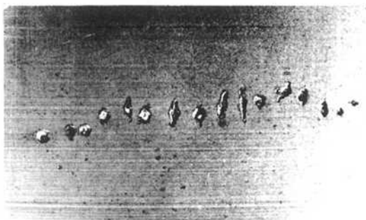
Figure 3-60. Electric pitting on surface of spherical outer raceway caused by the passage of a relatively large current.
