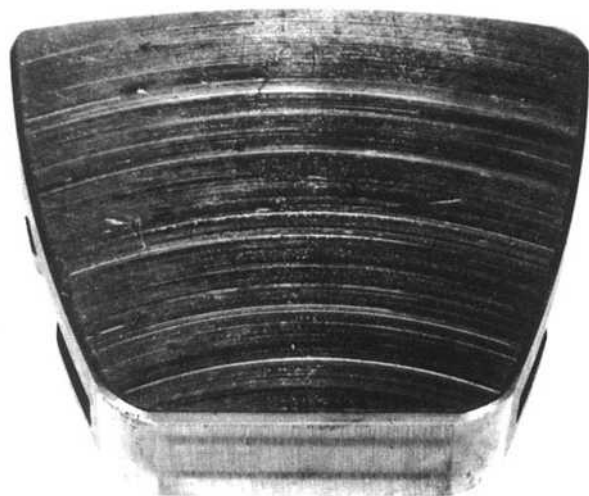
Figure 3-68. Concentric scoring due to dirt entering at high speed.
