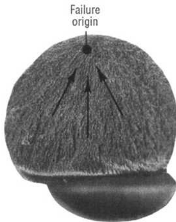
Figure 2-10. The chevrons or arrows on the face of a brittle fracture always point to the origin of a crack.
