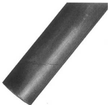
Figure 2-18. Jagged, detached, irregular cracks tend to indicate unusual metallurgical problems.
