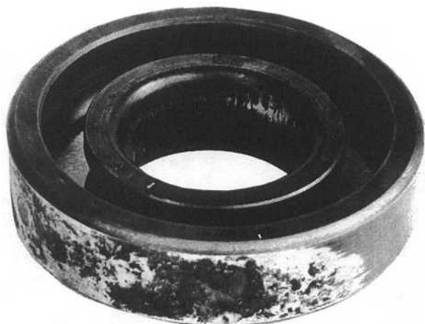
Figure 3-18. Wear due to fretting corrosion.
