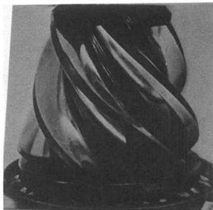
Figure 3-110. Polishing. Run-in under operating conditions, this hardened hypoid pinion has developed a highly polished surface. Undoubtedly the extreme-pressure additives in the lubricant had a tendency to promote polishing on the tooth surfaces.
