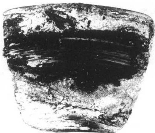
Figure 3-88. Thrust pad with severe "black scab" formation.
