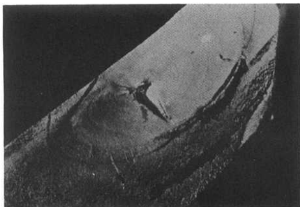
Figure 3-142. Fatigue Failure. This tooth fracture shows the “eye” and “beach marks” that typify a subsurface fatigue failure.
