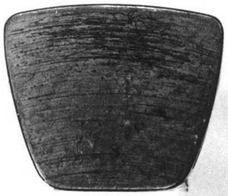
Figure 3-69. Dirt-intrusion damage at low-speed operation.
