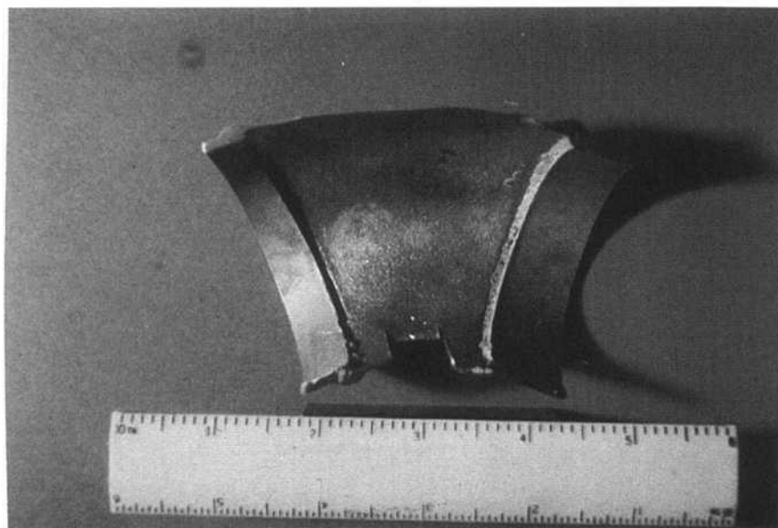
Figure 2-36. A 304L SS elbow mistakenly welded into a 316L piping unit. The elbow was actually stenciled 304L.
