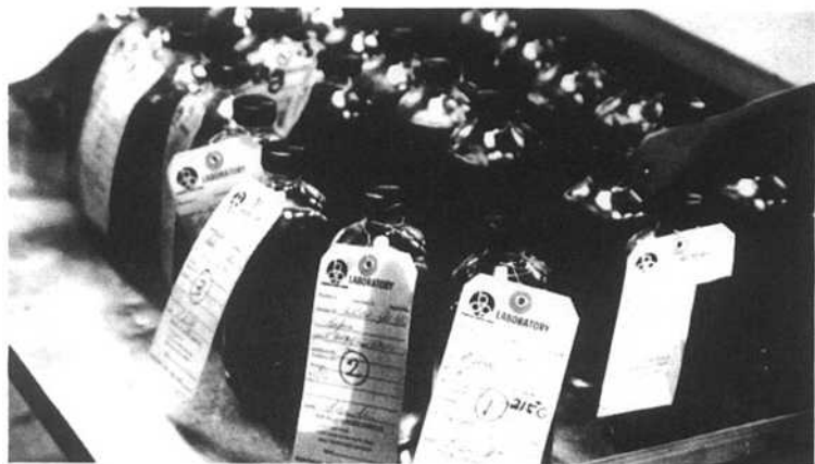
Figure 3-184. Lube-oil samples collected during the first two or three working days of each month.
