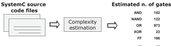
FIGURE 3.2: Complexity estimation from SystemC source code.
