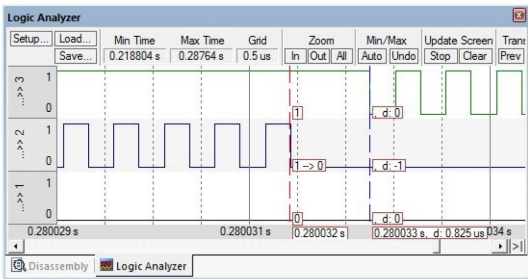
Figure 3.14. Profile showing the thread switch time is about 0.8 \mu s, measured in simulator for the TM4C123.
