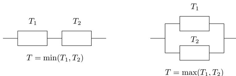
**Fig. 3.12** Systems in series and parallel.
