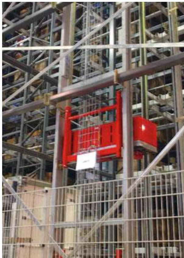
Gambar 8.6 AVSRS on an elevator returning from a higher-level tier after storing a pallet (Savoye Logistics).
