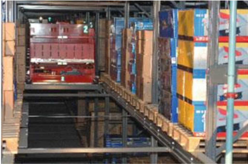
(a) AVSRS tunneling on rails (Savoye Logistics).
